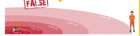
A sound level decreases by 6 decibels each time the distance from the source doubles. For example, with the disc cutter that emits 110 dB at 1 meter, you would need to be 32 meters away to find a sound level of 80 decibels.
